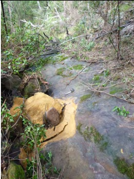
Photo 29: WCA5_LW38_001- upstream section of fracturing and dislodged rock, looking across stream. Taken on 24/04/2015
