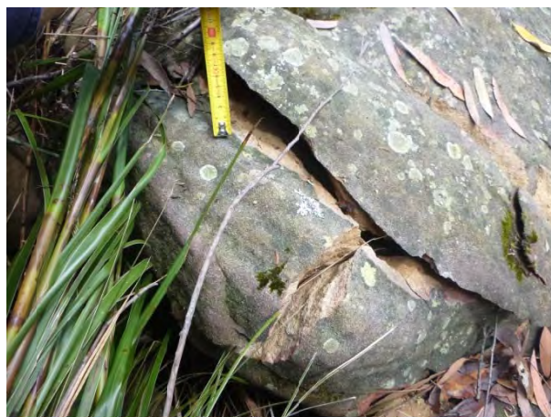
Photo 2: Impact WCA5_LW38_007- additional fracturing to boulder on GR110. Taken on 16/11/2015.
