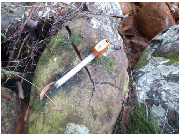
Photo 1: Impact WCA5_LW38_007- initial fracturing identified on tributary GR110. Taken on 2/10/2015.
