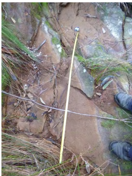
Photo 1 : WCA5_LW38_002 – Fracturing perpendicular to bedding plane. Taken on 03/08/2015.
