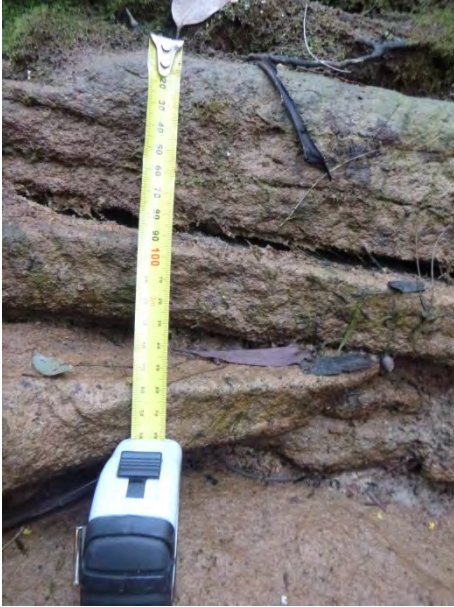
Photo 3: WCA5_LW38_002 – Extension along bedding plane. Taken on 03/08/2015
