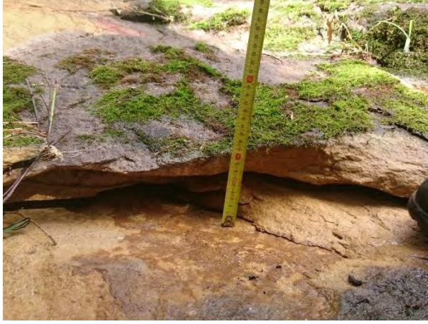
Photo 33: WCA5_LW36_001- fracturing to incised bedding plane. Taken on 24/04/2015
