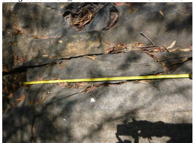
Photo 8: Impact WCA5_LW38_008- Displacement of pool bed rock material . Taken on 10/12/2015.
