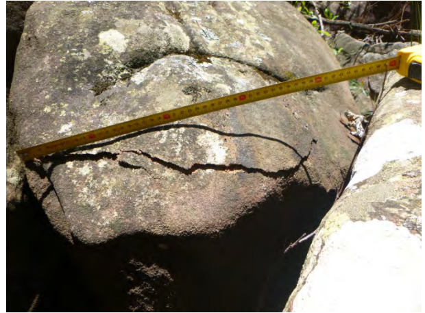
Photo 6: Impact WCA5_LW38_007- additional fracturing to boulder on GR110. Taken on 16/11/2015.
