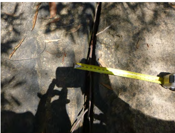
Photo 7: Impact WCA5_LW38_008- Debris infilling fracture on the base of GR_Pool 49. Taken on 10/12/2015.
