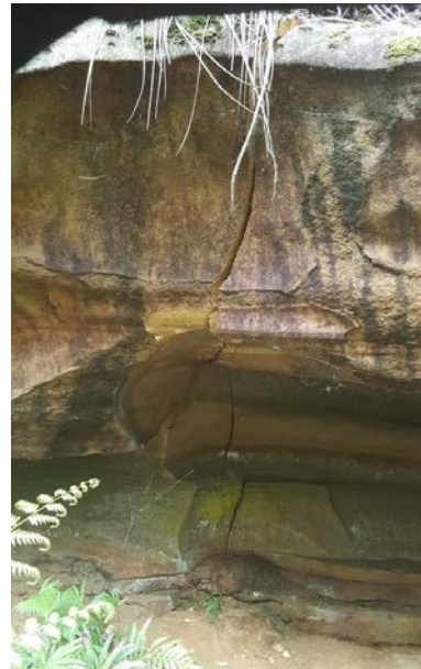
Photo 13: WCA5_LW38_010, Fracturing to rock outcrop adjacent to GR110. Taken on 17/02/16.
