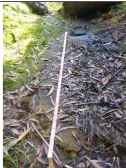
Photo 2: WCA5_LW36_001, fracturing and uplift of rock bed at GR104_Pool 1 looking northwest. Taken on 19/06/2014.
