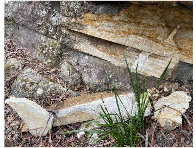
Photo 20: DA3B_LW18_018, Rock fracturing and rock fall, northern slope of LA2 valley. Taken 16/8/2022.
