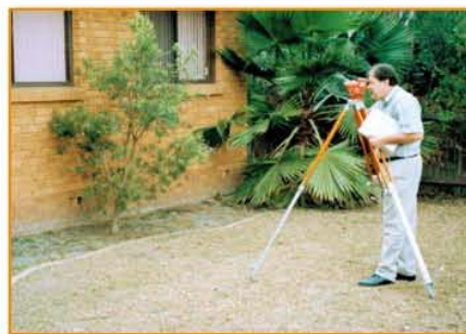
▼ Pre-mining inspections record any pre-existing damage.
