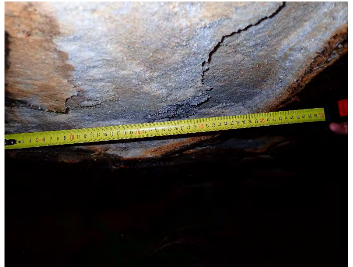
Photo 8: DA3C_LW21_016, underside of step from which rock fragments fell. Taken on 11/07/2023.
