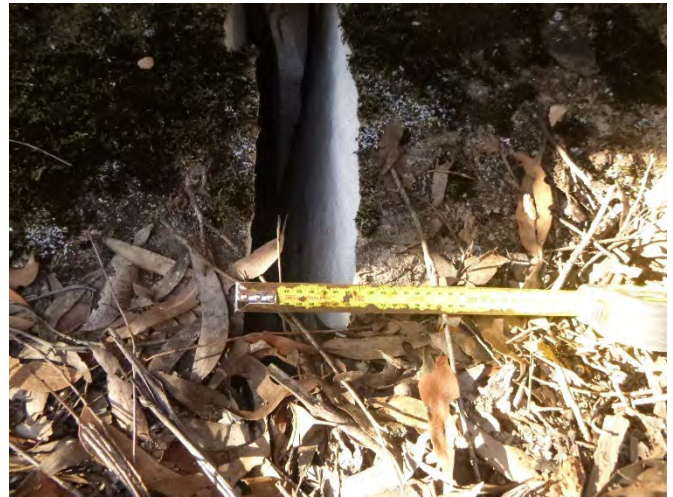
Photo 6: DA3C_LW21_007, maximum width of rock fracture. Taken on 15/06/2023.
