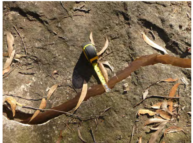
Photo 4: DA3C_LW21_006 , maximum width of rock fracture. Taken on 15/06/2023.
