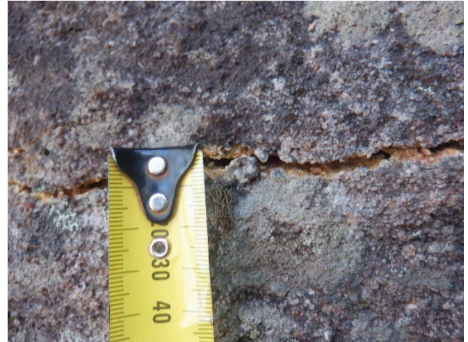
Photo 102: DA3C_LW21_028 , width of rock fracture. Taken 06/09/2023.
