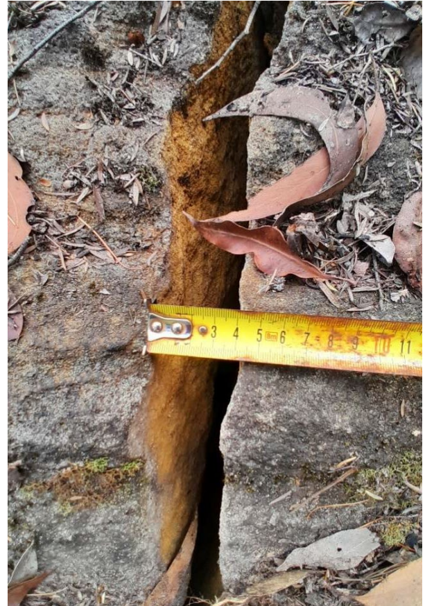
Photo 106: DA3C_LW21_030, width of rock fracture. Taken: 12/09/2023.
