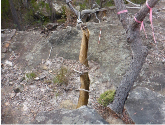
Photo 37: DA3C_LW21_002, showing largest rock fracture in series. Taken on 06/06/2023.
