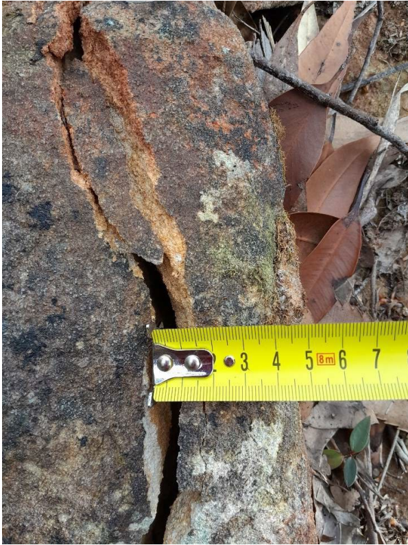
Photo 107: DA3C_LW21_031, width of rock fracture. Taken: 12/09/2023.
