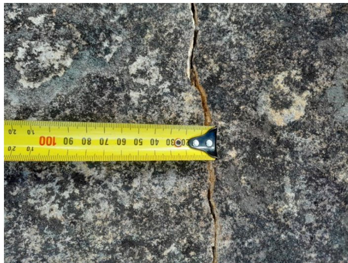
Photo 89: DA3C_LW21_023 , maximum width of the rock fracture. Taken: 31/08/2023.
