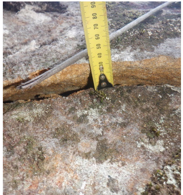
Photo 98: DA3C_LW21_026, Width of rock fracture. Taken 06/09/2023.
