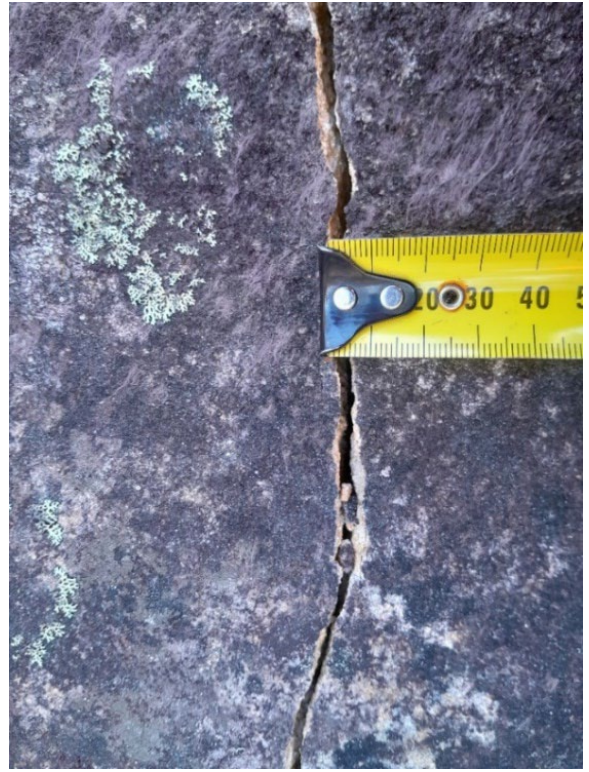
Photo 91: DA3C_LW21_024, maximum width of the rock fracture. Taken: 31/08/2023.
