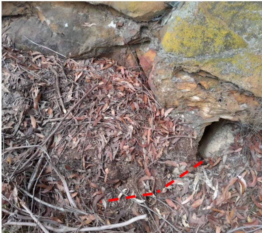
Photo 115: DA3C_LW21_034. Dashed line shows approximate section of unstable soil/leaf litter extending from rock movement. Taken 12/09/2023.
