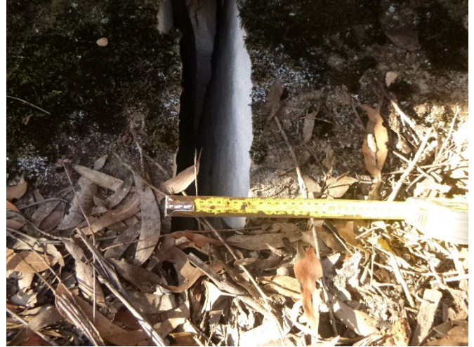
Photo 53: DA3C_LW21_007, maximum width of rock fracture. Taken on 15/06/2023.
