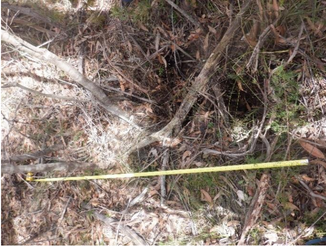
Photo 45: Maximum continuous length of soil cracking (measuring tape set at 2.5m). Taken 31/08/2022.
