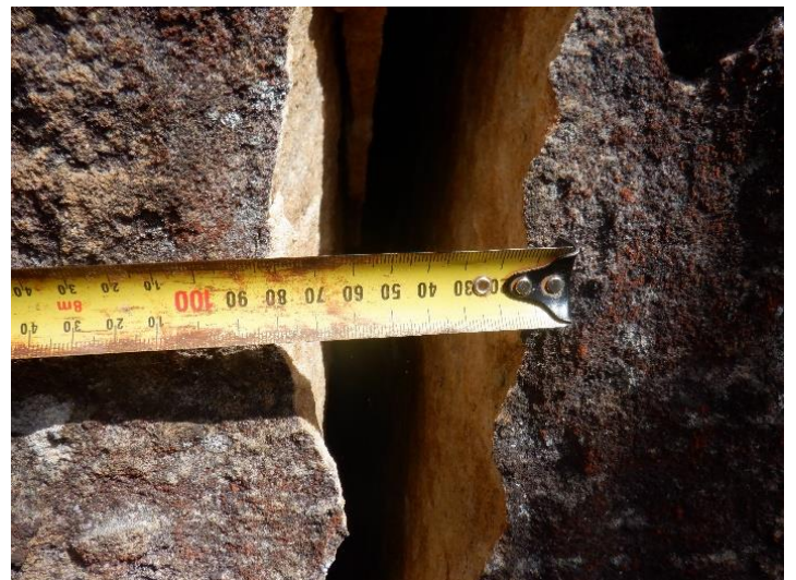
Photo 35: DA3A_LW19_001, showing width of rock fracturing. Taken 19/04/2023.
