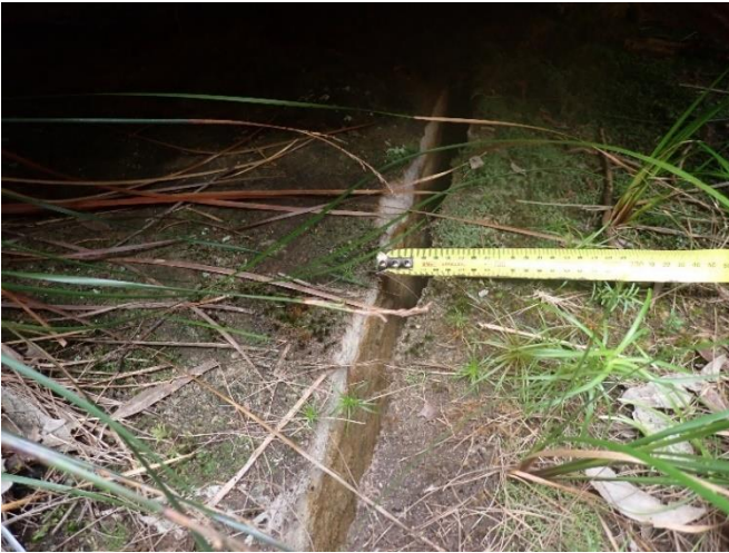
Photo 26: DA3A_LW8_003, looking at the width of rock fracturing. Taken 12/04/2023.
