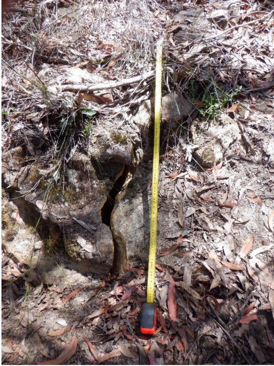
Photo 91: DA3A_LW19_023 , section of rock displacement. Taken on 13/12/2022.
