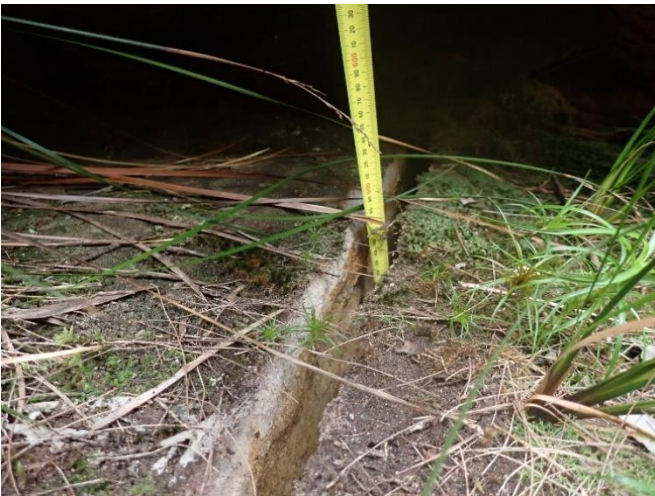
Photo 28: DA3A_LW8_003, looking at the depth of rock fracturing. Taken 12/04/2023.
