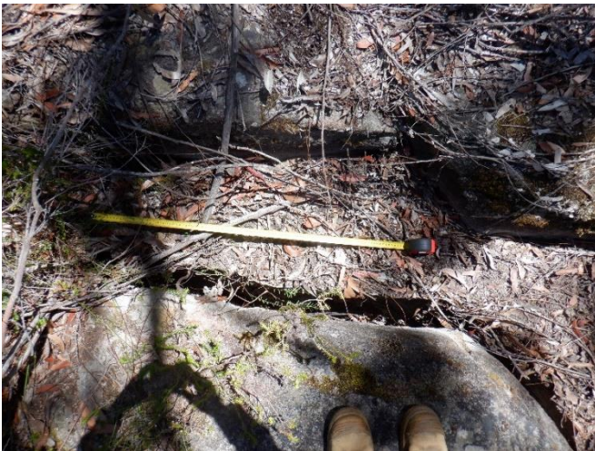
Photo 89: DA3A_LW19_022 , section of rock displacement. Taken on 13/12/2022.
