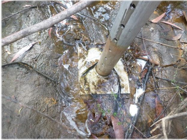
Photo 7: Flow diversion adjacent to monitoring equipment at LA4S1. Taken on 3/05/2017.
