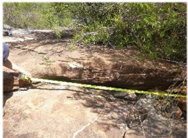
Photo 18: DA3B_LW13_022, looking upstream towards lateral fracturing on face of step. Taken 29 th March 2018.
