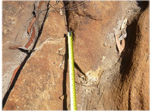
Photo 26: DA3B_LW13_035, looking across stream at the section of plating and uplift. Taken 23rd April 2018.
