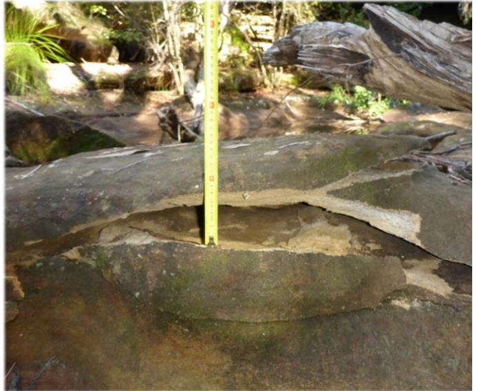
Photo 28: DA3B_LW13_040, looking at a section of rock uplift. Taken 7 th May 2018.
