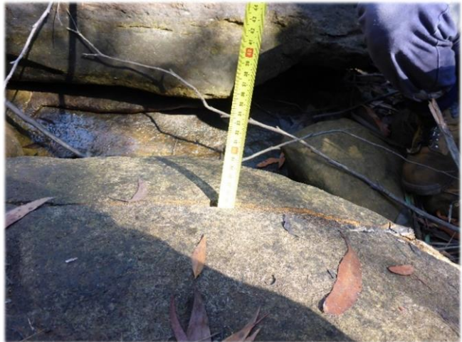
Photo 30: DA3B_LW13_040, looking at the maximum measurable depth of the rock fracturing. Taken 7 th May 2018.
