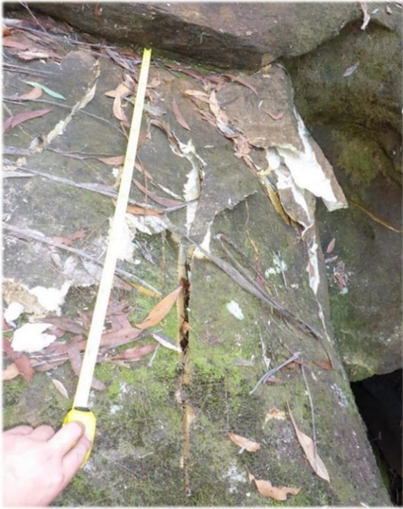
Photo 27: DA3B_LW13_040, looking at a section of rock fracturing and uplift. Taken 7 th May 2018.
