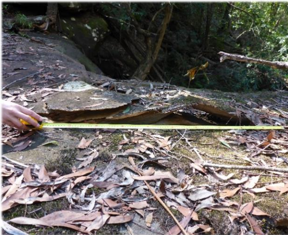
Photo 29: DA3B_LW13_040, looking at a section of rock fracturing and uplift. Taken 7 th May 2018.
