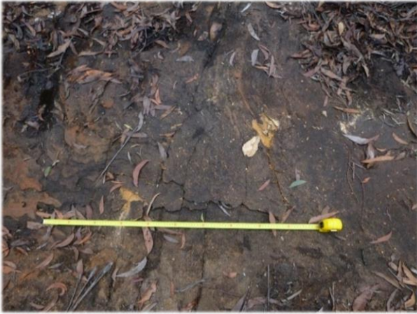
Photo 36: DA3B_LW13_042 , looking at a section of rock fracturing and uplift. Taken 16th May 2018.
