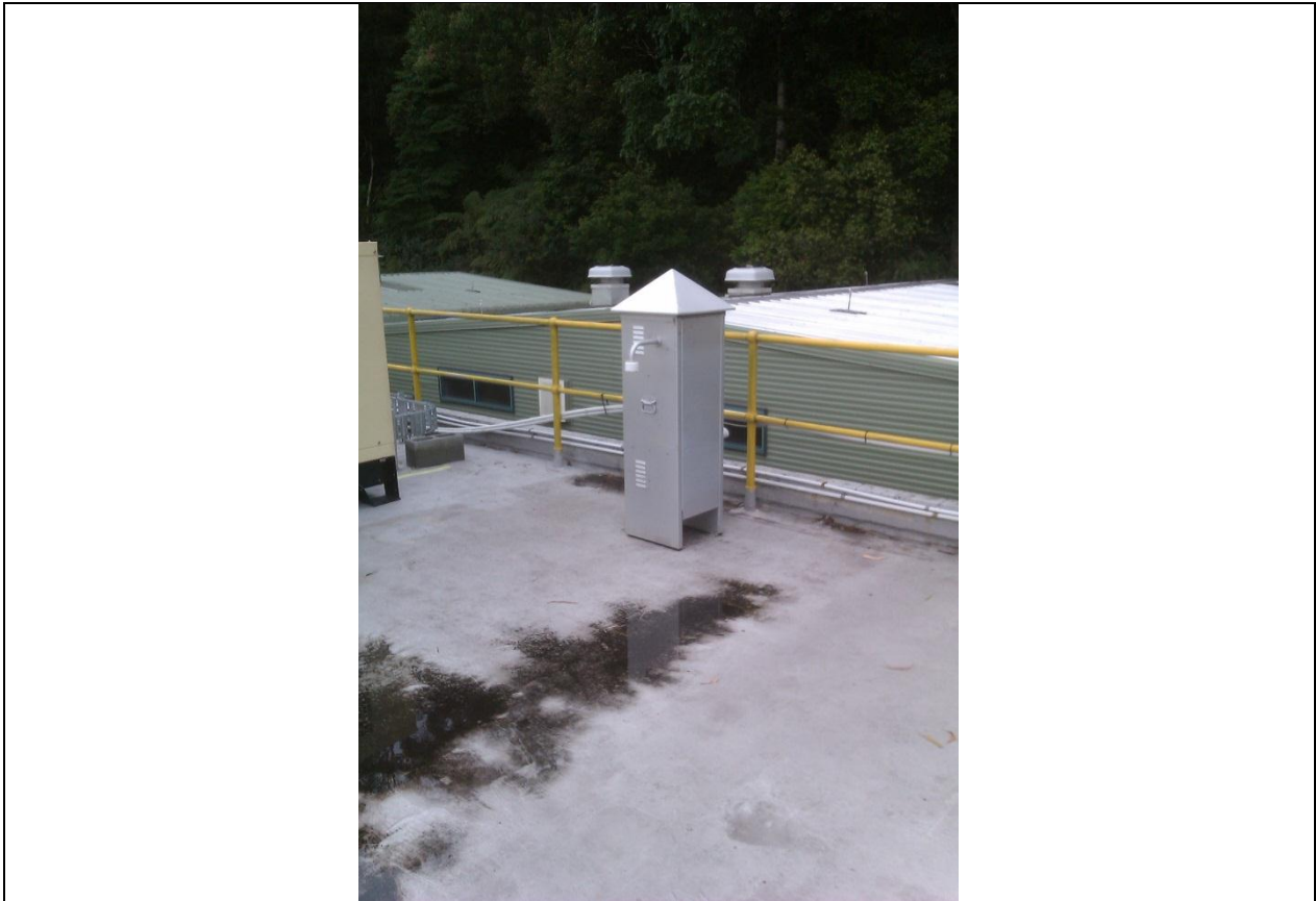
Picture A5: High Volume Air Sampler Point 21 with TSP sampling head - located on top of the bathhouse building, Pit Top
