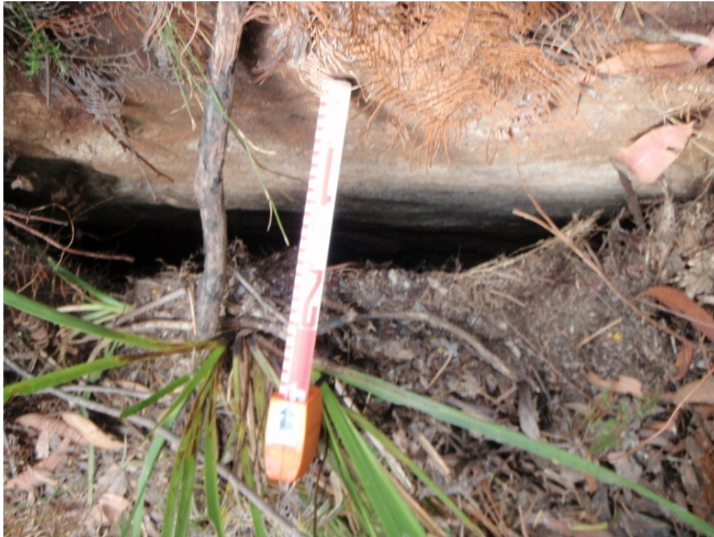
Photo 4 - Typical Area 3A Surface Crack in Near Surface Sandstone Outcrops
