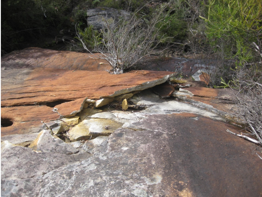
Photo 1 - Down stream Rock Bar Cracking and Iron staining along 1st Order Creek No. SC10C, Area 3A (>2 years since mining of LW 7)
