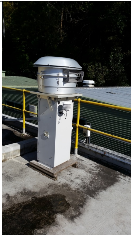
Picture E4: High Volume Air Sampler Point 21 with PM 10 sampling head - located on top of the bathhouse building, Dendrobium pit top
