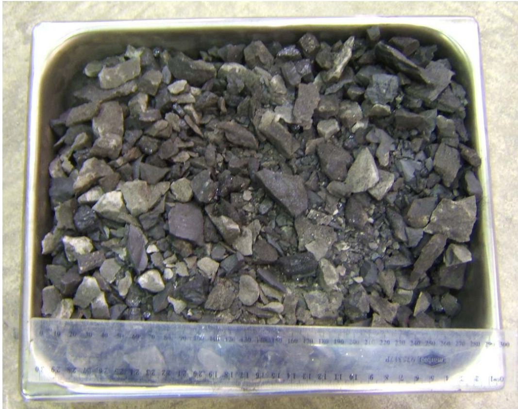
Figure 1: Crushed coal wash aggregate.
