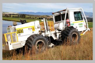
Vibroseis Truck uses low-frequency vibrations to analyse underground geology along seismic lines.
