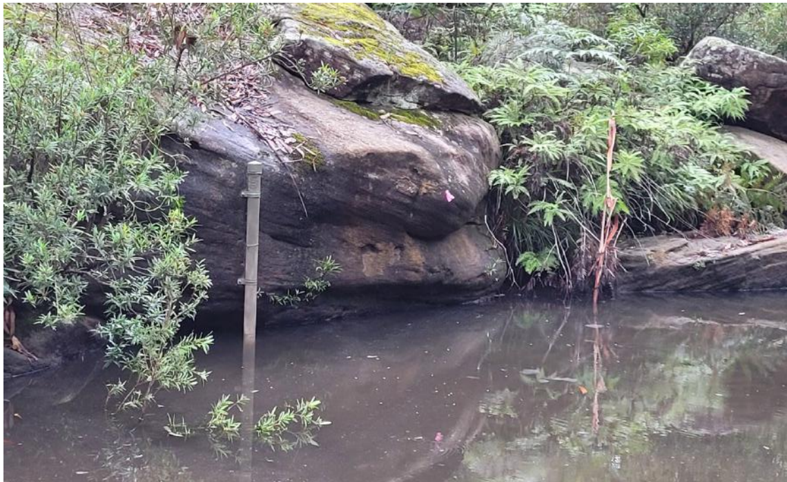
Plate 7: Water level logger installed in Georges River monitoring site Point 11
