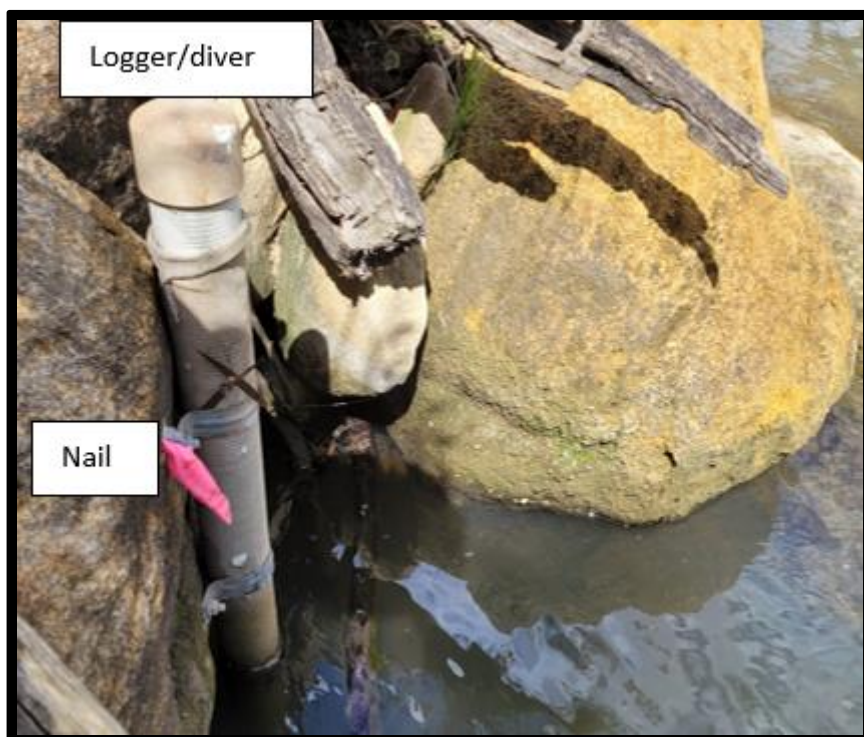
Figure 5. Water level field sampling equipment
