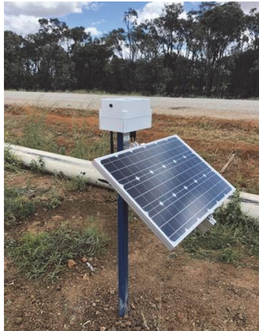
Fig. 6.5 Nominal GNSS unit installation set-up
