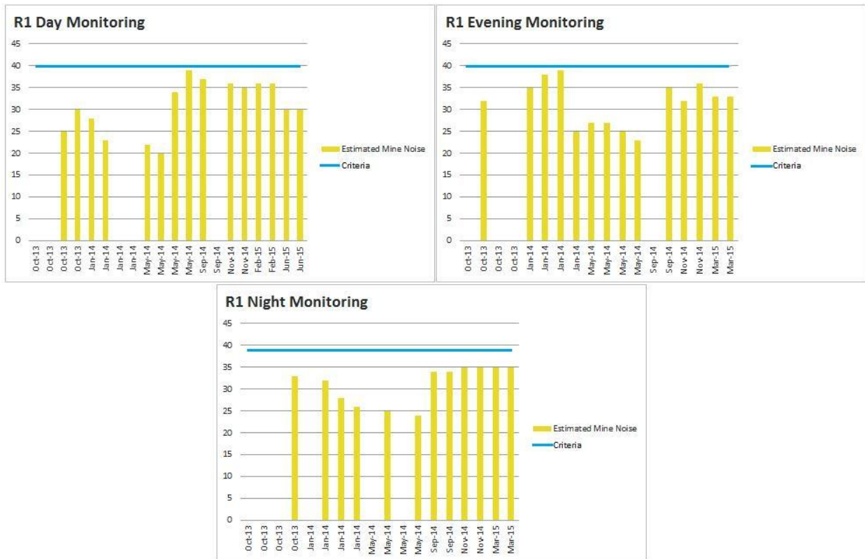
Figure 11: Site R1 Noise Compliance (LAeq, 15 minute) during the Reporting Period
