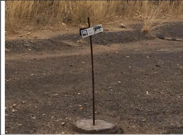
Figure 7: Prospecting Test Borehole (sealed)
