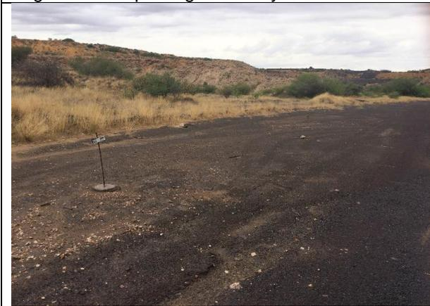
Figure 5: Prospecting Test Borehole (sealed)
