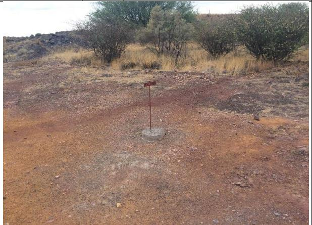
Figure 10: Prospecting Test Borehole (sealed) with remnants of vegetation clearing
