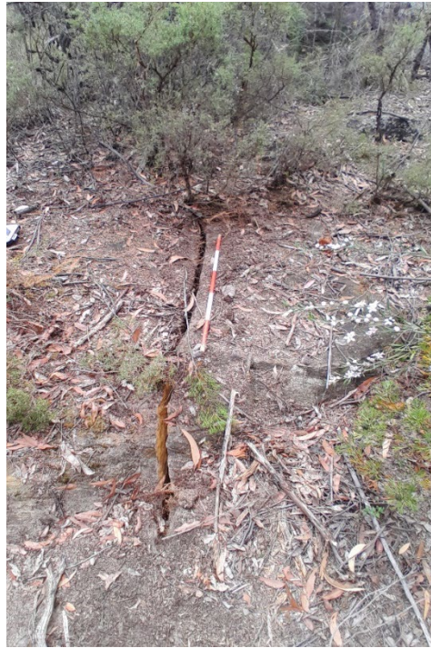
Photo 33: DA3C_LW21_030 , overview of rock fracture. Taken: 12/09/2023.
