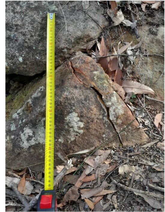
Photo 34: DA3C_LW21_031 , overview of rock fracture. Taken: 12/09/2023. Note - measurement tape set to 0.5m for scale.
