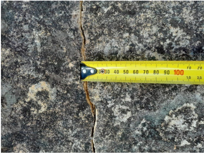
Photo 26: DA3C_LW21_023 , maximum width of the rock fracture. Taken: 31/08/2023.
