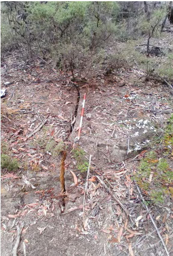
Photo 1: DA3C_LW21_030 , overview of rock fracture. Taken: 12/09/2023.
