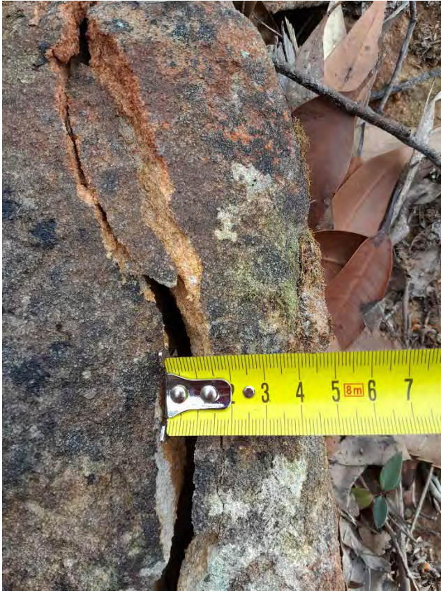
Photo 3: DA3C_LW21_031, width of rock fracture. Taken: 12/09/2023.
