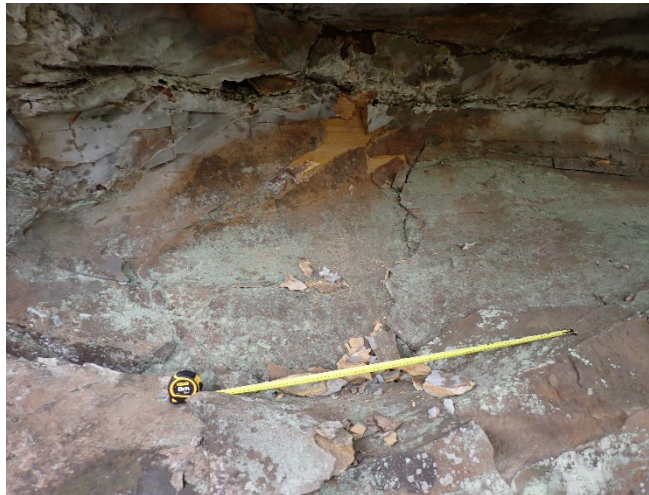
Photo 41: DA3A_LW19_042, showing rockfall and fragmentation at landscape monitoring site LW19_SS4. Taken on 12/04/2023.
