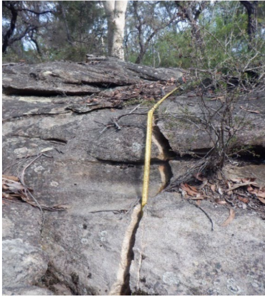
Photo 7: DA3A_LW19_001 showing rock fracturing. Tape set at 2m. Taken on 19/04/2023.
