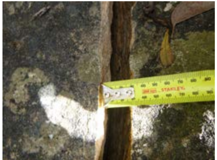
Photo 2: DA3A_LW19_030, width of rock fracturing on outcrop. Taken on 15/2/2023.
