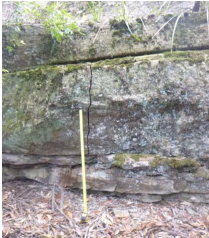
Photo 5: DA3A_LW19_032 , rock fracturing on side of outcrop. Taken on 15/2/2023
