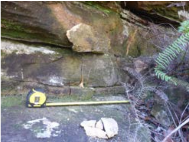
Photo 15: DA3A_LW19_058 , showing step where rock has detached from rock face. Taken on 5/05/2023. Note: Tape measure is set to 0.5m in length.
