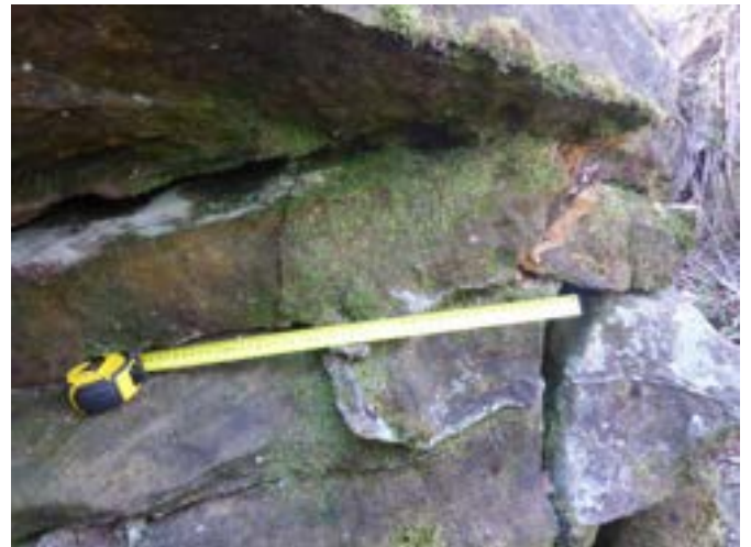
Photo 16: DA3A_LW19_058 , showing step where rock has detached from rock face. Taken on 5/05/2023. Note: Tape measure is set to 0.5m in length.
