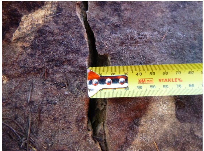
Photo 2: DA3B_LW18_007 , showing the width of rock fracturing. Taken 8/06/2022.
