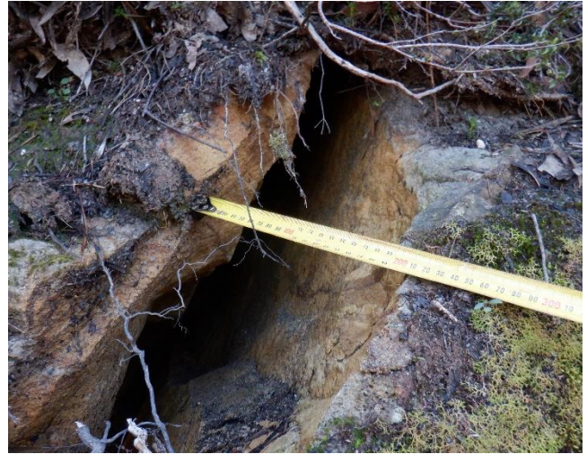
Photo 4: DA3B_LW18_014, maximum width of fracture. Taken 16/08/2022
