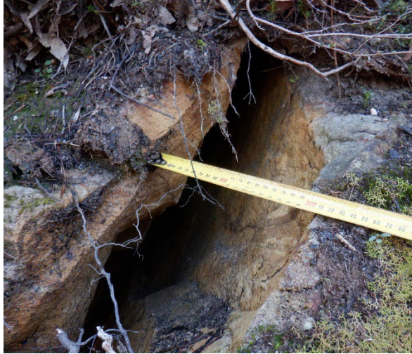
Photo 52: DA3B_LW18_014 , maximum width of fracture. Taken 16/08/2022
