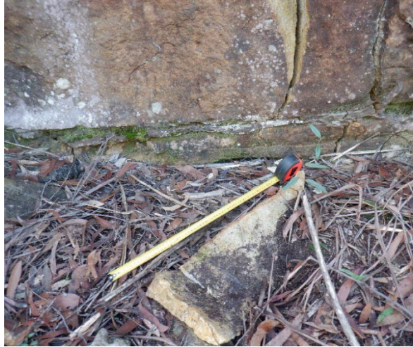
Photo 50: DA3B_LW18_013 , showing rock fragmentation. Taken 16/08/2022.
