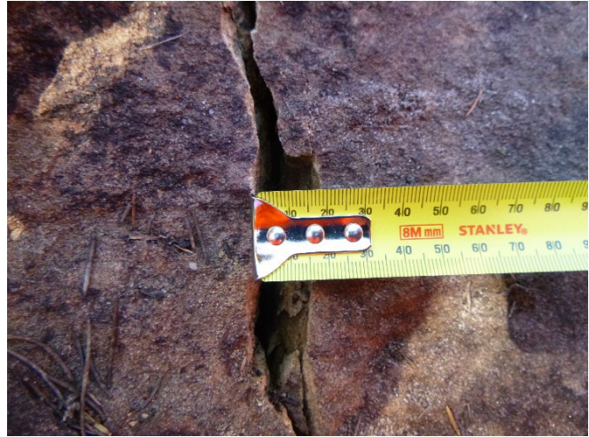
Photo 36: DA3B_LW18_007 , showing the width of rock fracturing. Taken 8/06/2022.
