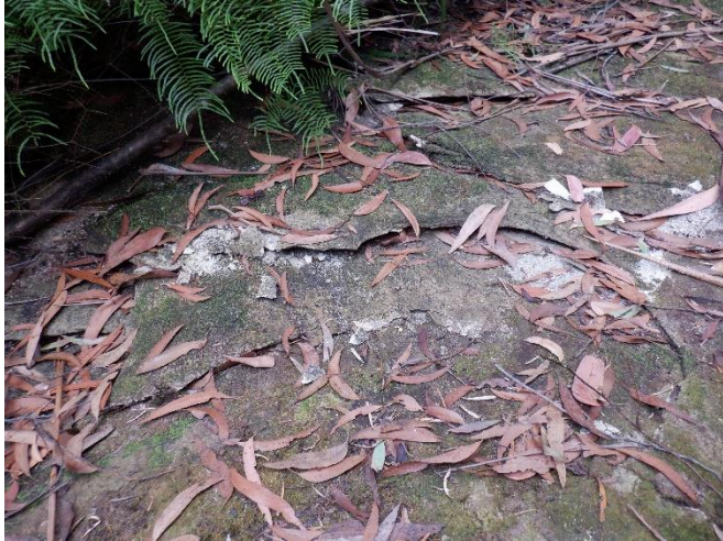
Photo 7: DA3B_LW17_007 , section of rock fracturing on LA2. Taken on 10/03/2021.
