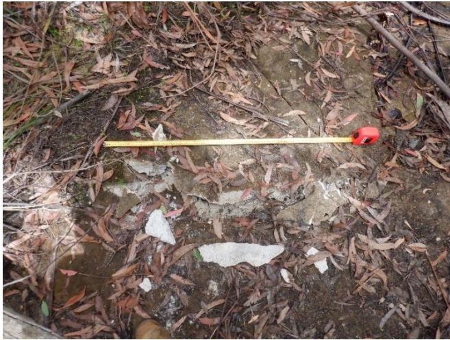
Photo 1: DA3B_LW17_001, rock fracturing, uplift and fragmentation on rockbar. Taken on 5/02/2021.
