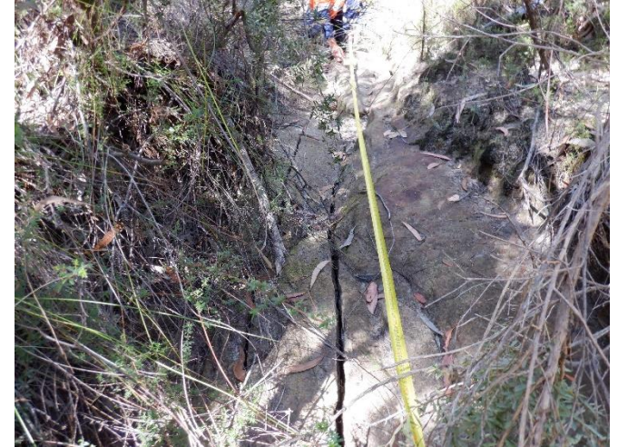
Photo 9: DA3B_LW17_013 , rock fracturing on LA2. Taken on 13/04/2021.
