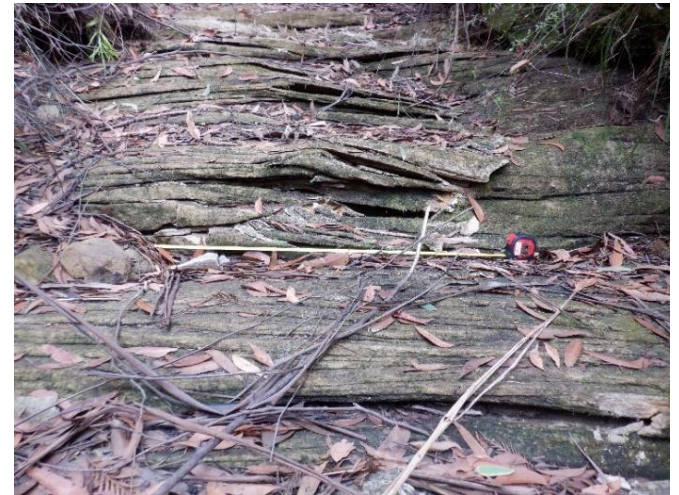
Photo 6: DA3B_LW17_006, rock fracturing and uplift on LA2. Taken on 10/09/2021.
