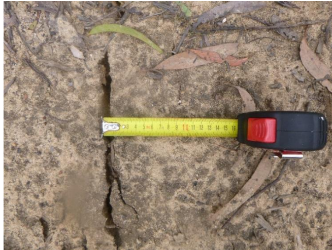
Photo 36: DA3B_LW17_028 , soil cracking on access track. Taken on 26/07/2021.
