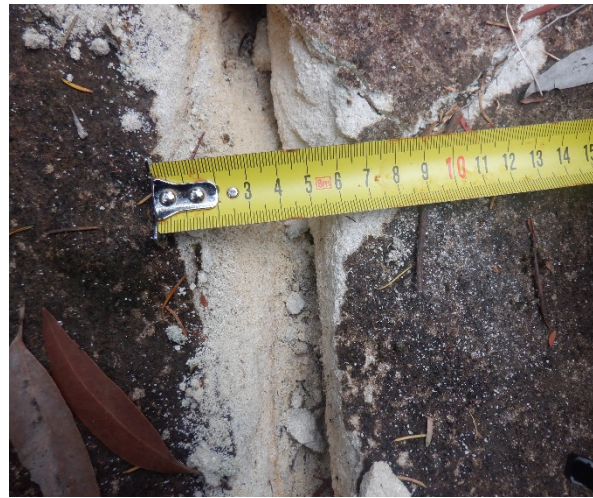
Photo 10: DA3B_LW17_004, looking at the maximum width of the rock fracturing. Taken on 10/03/2021.
