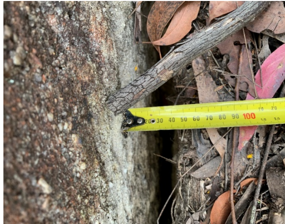
Photo 97: DA3B_LW17_038, looking at a section of rock displacement, showing the width. Taken 15/9/2021.
