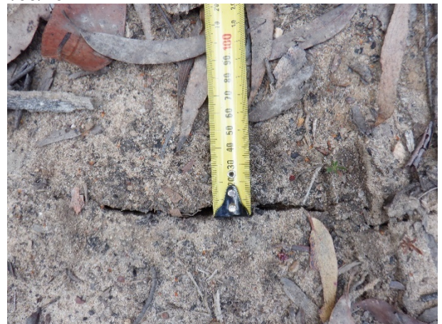
Photo 120: DA3B_LW17_030- soil cracking on Fire Road 6A has been remediated, soil cracking to the side of the fire road remains. Taken on 21/09/2021.
