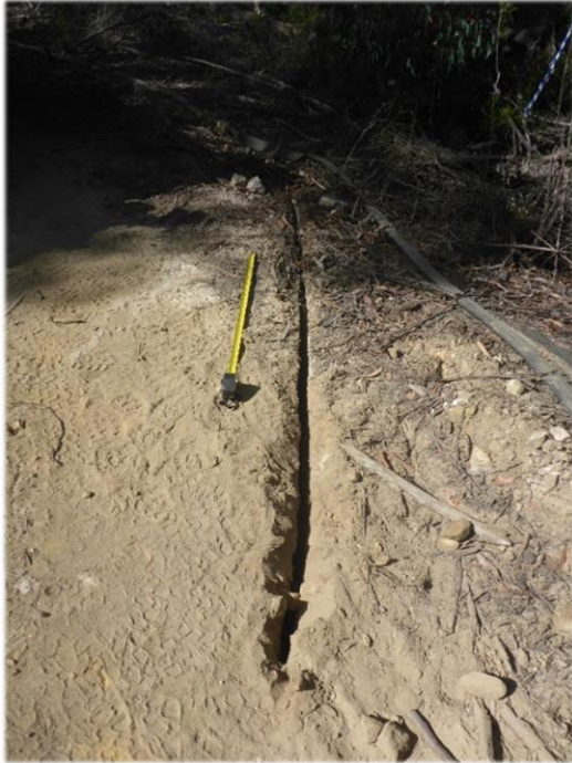
Photo 34: DA3B_LW16_003 , soil cracking and rock fracturing on access track between Lake Avon and FR6A . Taken on 22/04/2020.
