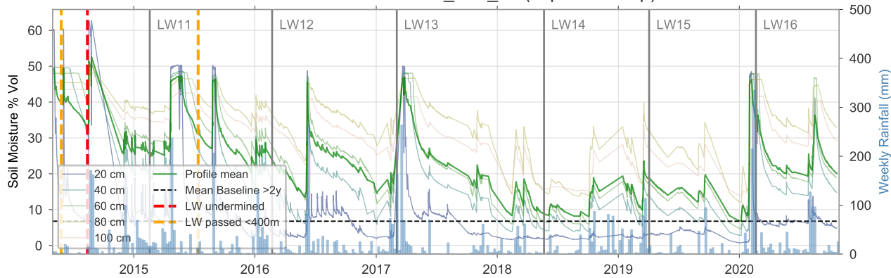
Soil moisture sensor S08_S05 (impact swamp)
