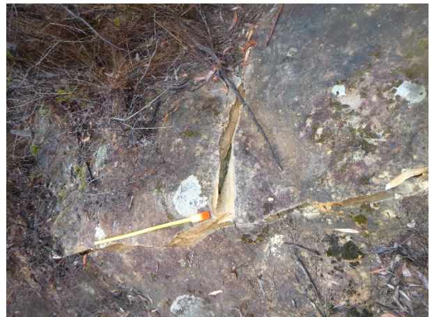
Photo 18: DA3B_LW14_019, looking at a section of rock fracturing and uplift. Taken on 9/09/2020.
