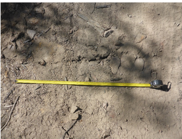
Photo 109: DA3B_LW16_007, soil cracking on access track between Lake Avon and FR6A. Taken on 22/04/2020.
