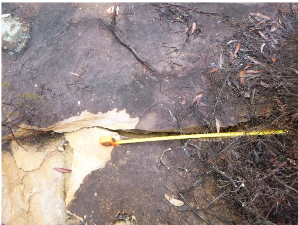
Photo 17: DA3B_LW14_019, looking at a section of rock fracturing and displacement. Taken on 9/09/2020.
