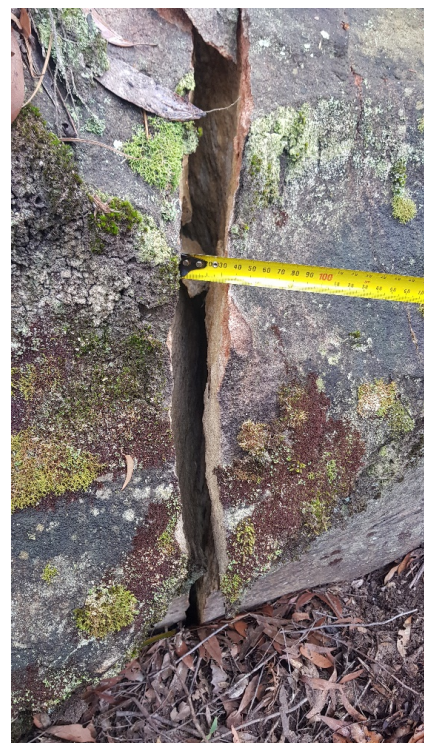
Photo 29: DA3B_LW16_012, looking at the maximum width of the rock fracture. Taken on 28/04/2020.
