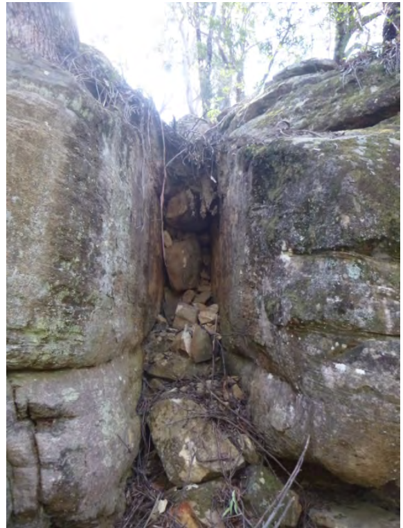
Photo 7: DA3B_LW16_029- rockfall from step, looking at top of step where fragment originated. Taken on 31/08/2020.
