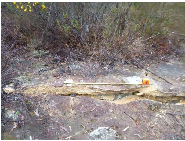
Photo 5: DA3B_LW14_019, looking at a section of rock fracturing and uplift. Taken on 9/09/2020.
