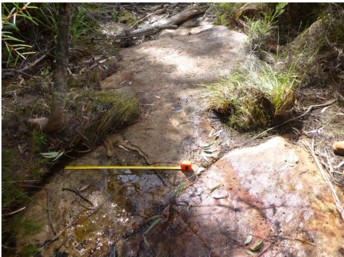
Photo 1: DA3B_LW16_028- rock fracture in foreground and edge of dry step and Pool 34 in background. Taken on 31/08/2020.
