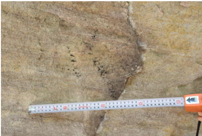
Plate 14: Slight opening of bedding plane adjacent to Art Panel located in the southern extent of the shelter.
