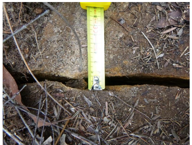
Photo 10: DA3B_LW15_014 , looking at widest rock fracture. Taken on 11/10/2019.
