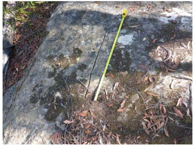
Photo 8: DA3B_LW14_025 , looking at a section of the rock fracturing. Taken 09/04/2019.
