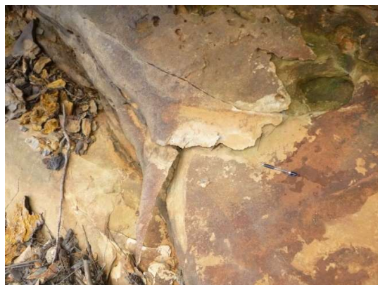
Photo 2: DA3B_LW13_043, looking at a section of rock fracturing and uplift. Taken on 6 December 2018.
