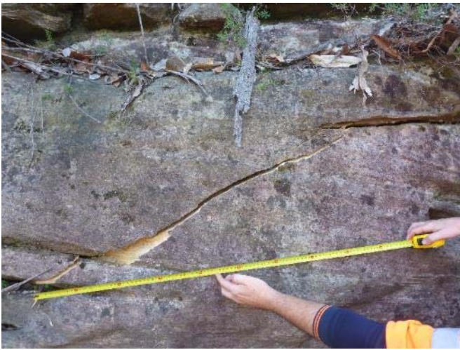
Photo 7: DA3B_LW14_025 , looking at a section of the rock fracturing and displacement. Taken 09/04/2019.
