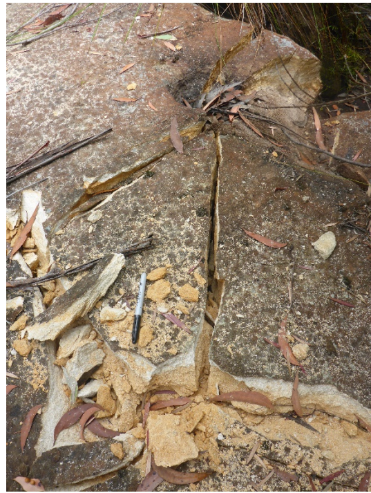
Photo 7: Fracturing and dislodged sections of rock extending along rockbar. Taken on 21/01/2019.
