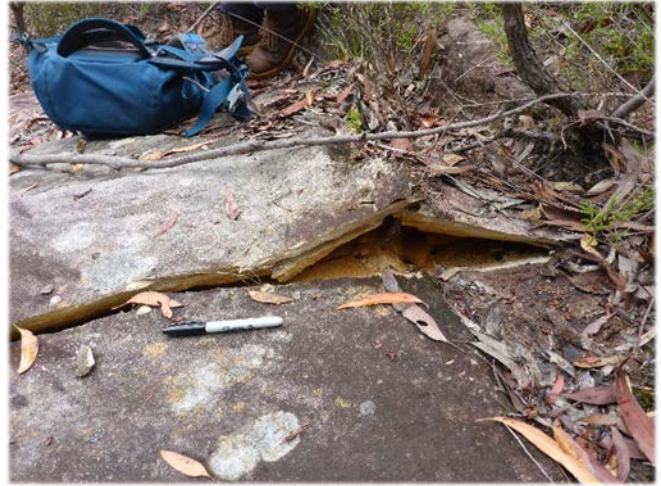
Photo 30: DA3B_LW13_035, fracturing and uplift on rockbar. Taken on 21/01/2019.
