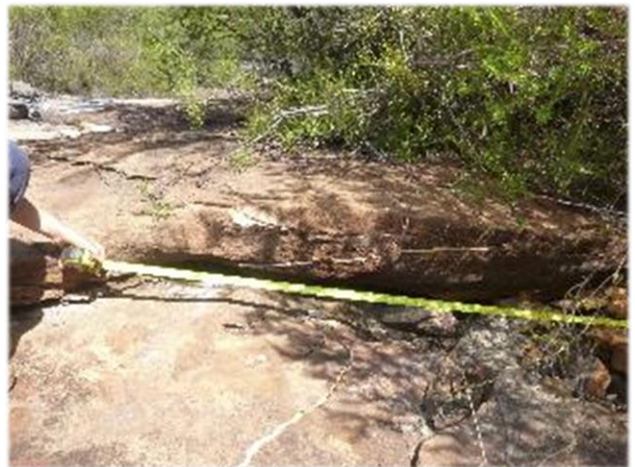
Photo 14: DA3B_LW13_022, looking upstream towards lateral fracturing on face of step. Taken 29th March 2018.
