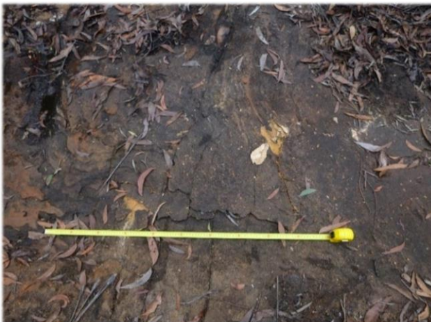
Photo 32: DA3B_LW13_042, looking at a section of rock fracturing and uplift. Taken 16 th May 2018.
