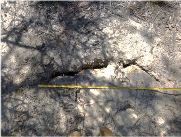
Photo 59: DA3B_LW13_032, soil cracking across Fire Road 6P. Taken 9th April 2018.
