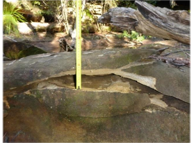
Photo 24: DA3B_LW13_040, looking at a section of rock uplift. Taken 7 th May 2018.
