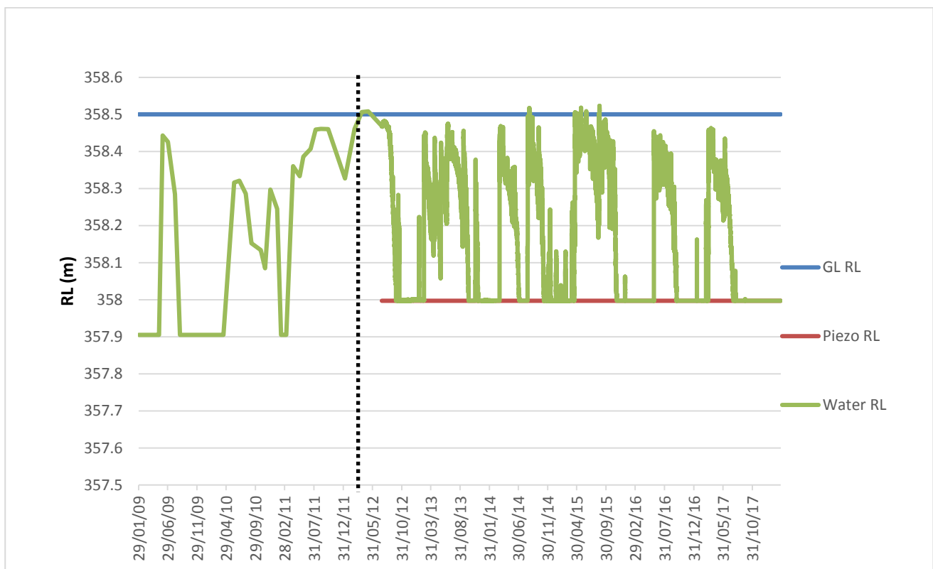
Figure 26 Swamp 15A Piezometer 15a_18 data (supplied by Illawarra Coal). Mining within the RMZ occurred in October 2012 (dashed vertical line).
