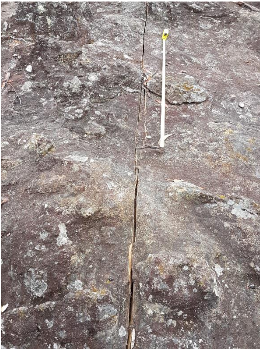
Photo 7: DA3B_LW12_026 - Fracturing to rock outcrop. Taken on 20/01/2017
