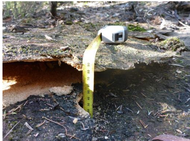
Photo 10: DA3B_LW12_008 – Uplift on Rockbar upstream of the basal step of Swamp 4. Taken on 20/05/2016.
