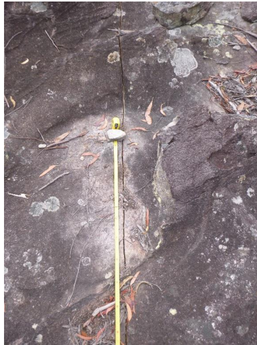
Photo 8: DA3B_LW12_026 - Additional fracturing to sandstone outcrop. Taken on 03/02/2017
