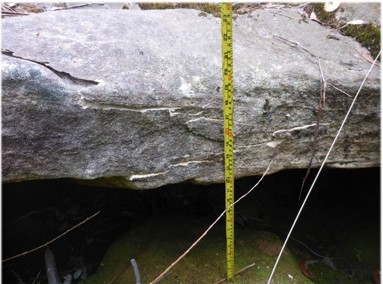
Photo 15: DA3B_LW12_019 – Fracturing to the face of a step in WC21_Step 48. Taken on 9/11/2016.
