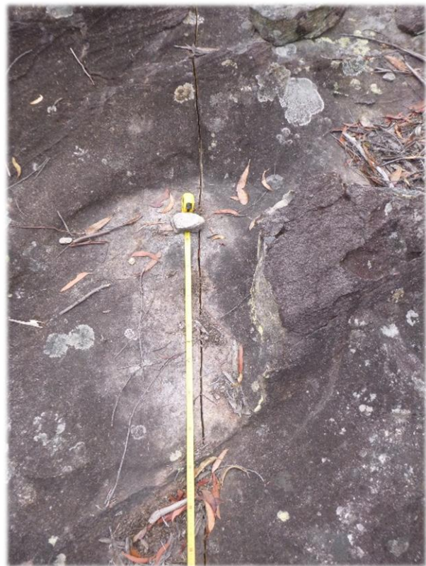
Photo 17: DA3B_LW12_026 - Additional fracturing to sandstone outcrop. Taken on 03/02/2017.
