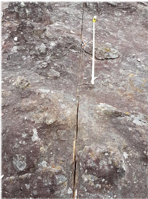
Photo 16: DA3B_LW12_026 - Fracturing to sandstone outcrop. Taken on 20/01/2017.
