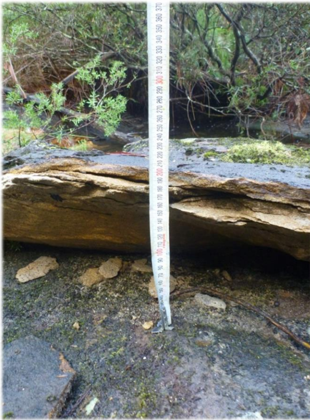
Photo 6: DA3B_LW12_005- Uplift and fracturing with fresh rock Photo 7: DA3B_LW12_005- Separated rock fragment. Taken on surface due to movement of rock fragments downstream. Taken on 5/07/2016. on 5/07/2016.
