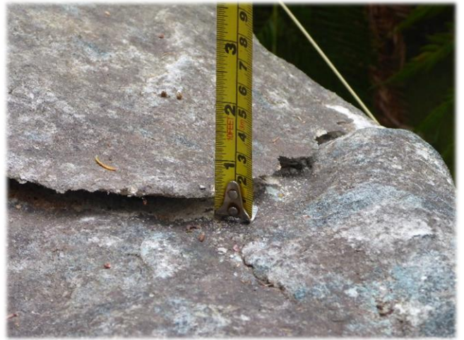
Photo 14: DA3B_LW12_019 - Highest section of uplift. Taken on 9/11/2016.
