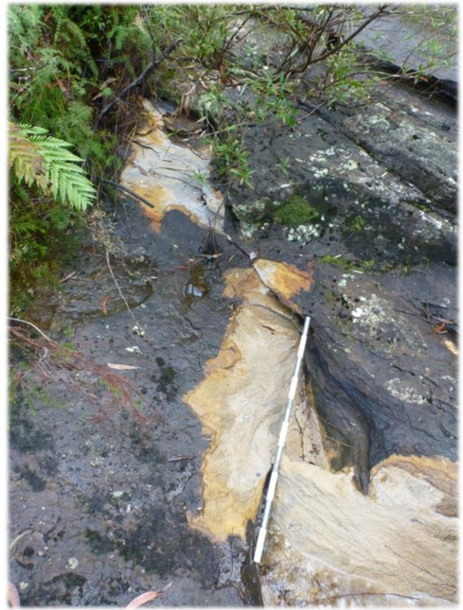
Photo 6: DA3B_LW12_005- Uplift and fracturing with fresh rock Photo 7: DA3B_LW12_005- Separated rock fragment. Taken on surface due to movement of rock fragments downstream. Taken on 5/07/2016. on 5/07/2016.
