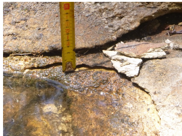
Photo 8: DA3B_LW11_010- Rock fracture and uplift, looking across stream along WC21. Taken on 11/02/2016.
