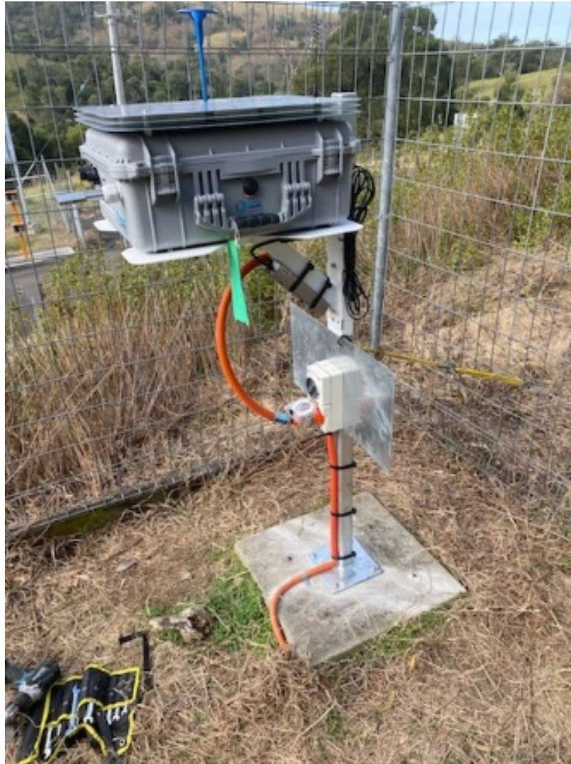
Plate 2: Photometer dust monitor located at the KVCLF
