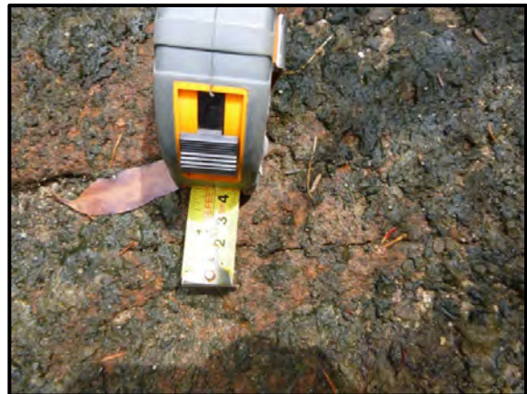
Photo 85: Impact DA3B_LW10_015- Fracturing downstream from WC21_Pool 23. Photo taken on 4 December 2014.
