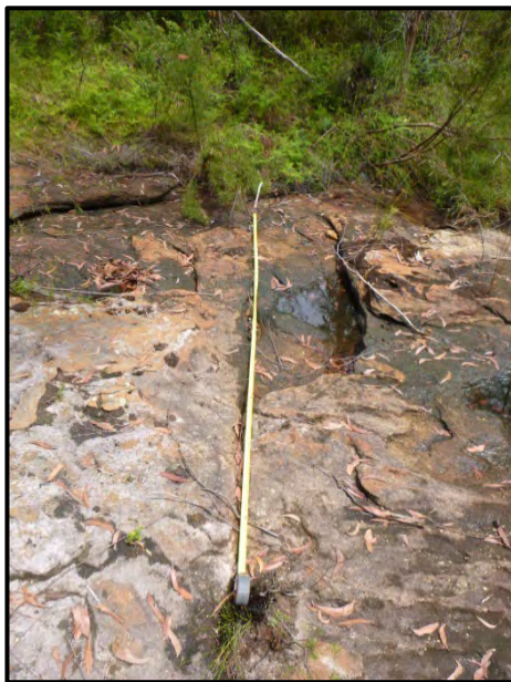
Photo 96: Impact LW10_016- Rock fracture extending across rockbar and through joint, looking across stream. Taken on 4 December 2014.
