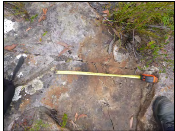
Photo 100: Impact LW9_022- Rock fracturing to Rockbar 18. Taken on 2 January 2014.
