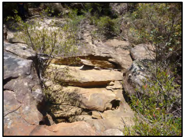
Photo 112: Impact DA3B_LW9_015- fracturing to base of WC21_Pool 16, looking downstream. Taken on 15 October 2015.
