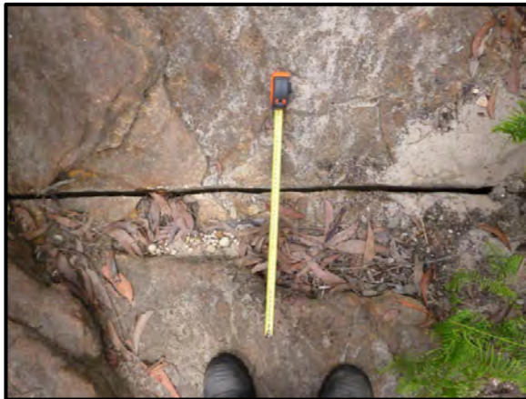
Photo 99: Impact LW9_021- Rock fracturing to Rockbar 18. Taken on 2 January 2014.
