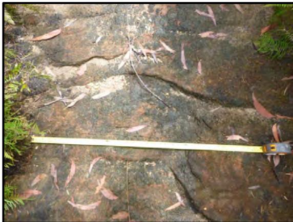
Photo 84: Impact DA3B_LW10_015- Fracturing downstream from WC21_Pool 23, looking upstream. Photo taken on 4 December 2014.
