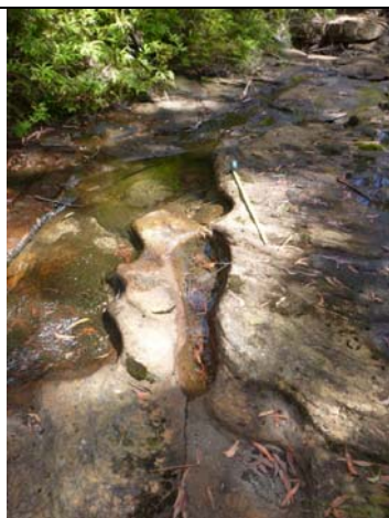
Photo 16: Impact LW10_020- fracturing to downstream end of Rockbar 24, looking downstream. Taken on 30/01/2015.
