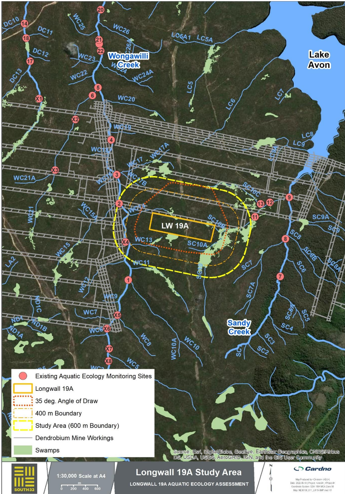
Figure 3-1 Aerial image overlaid with longwall layouts, watercourses and aquatic ecology sites within and adjacent to the Longwall 19A Study Area (600 m boundary). The 400 m boundary is presented to provide context for the subsidence predictions (Fracturing has been observed up to approximately 400 m outside of previously extracted longwalls in the Southern Coalfield (MSEC 2022).
