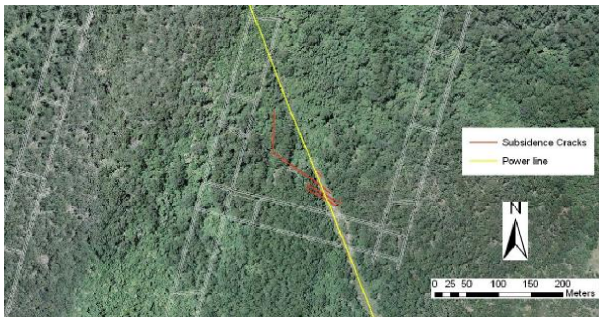
Fig. 5.20 Locations of Observed Surface Cracking above Longwall 3 in Area 2
