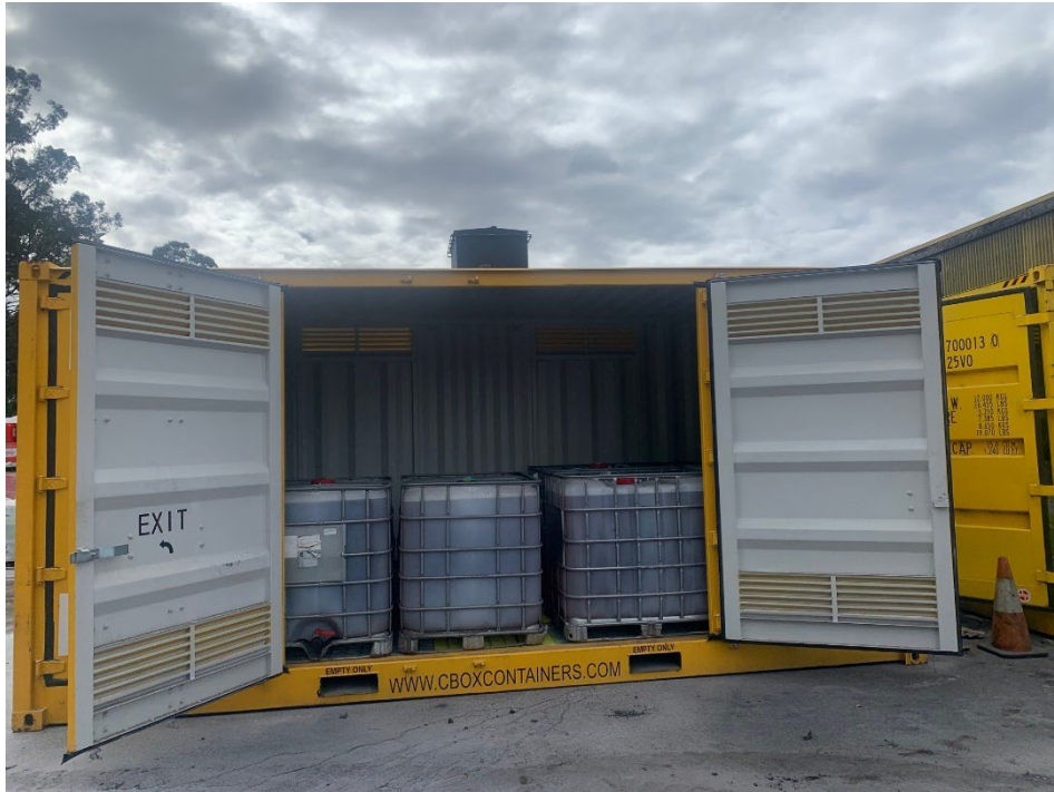
Plate 2: Self Bunded Storage Container
