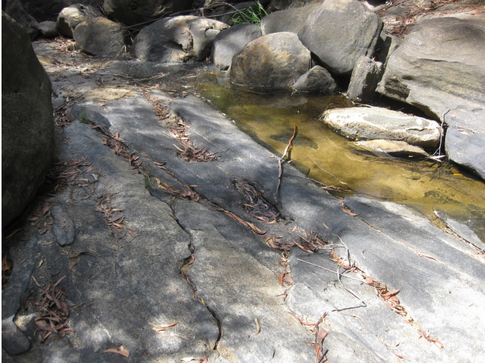
Photo 6 - Minor Rock Fall from Overhang along Georges River due to LW 35
