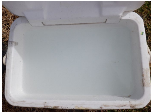
Photo 10: Closeup of water sample taken from borehole via pump. Very cloudy water with white/grey colour is visible in water sampled from borehole. Taken on 26 August 2022.
