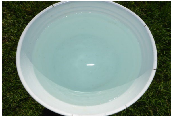
Photo 2: Water from GW110671, collected into a bucket. Samples and field parameters were taken from the bucket, photo taken on 15 November 2017.
