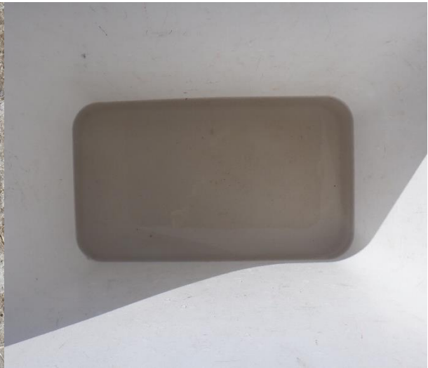
Photo 6: Closeup of water sample taken from borehole via bailing from borehole. Slight dark-brownish colour is visible in water sampled from borehole. Taken on 3 May 2021.
