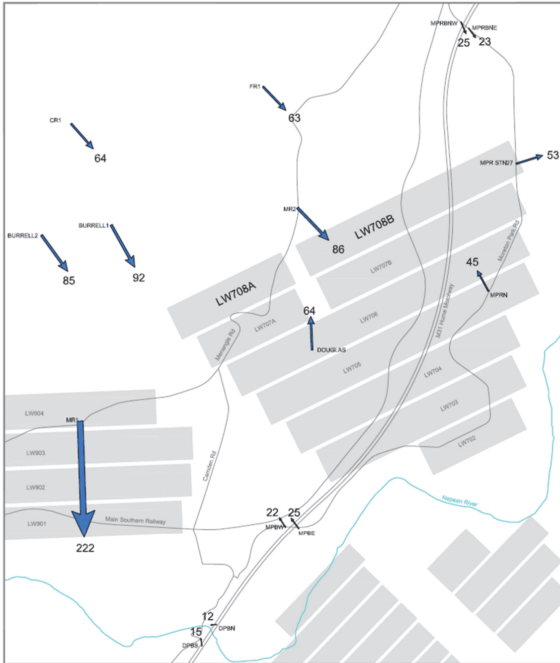
Fig. 2.4 Measured absolute incremental horizontal movements at the far-field 3D marks due to the mining of LW708A and LW708B
