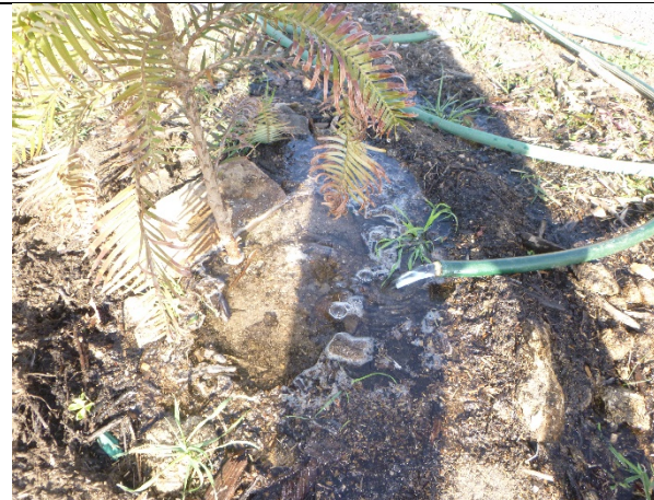
Photo 2: Borehole outlet purging during post-mining inspection. Taken on 25 th July 2018.
