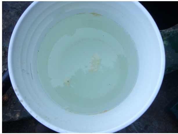
Photo 4: Collection of water from the holding tank with presence of orange film. Photo taken on 7/3/16.
